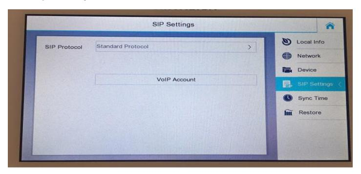
After device reboot, go to **Setting-> Configuration-> SIP Setting** and click VoIP Account, and input SIP server information.
