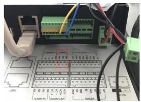
You can find the RS485 cable on the villa door station. (DS-KV8102-VP)
