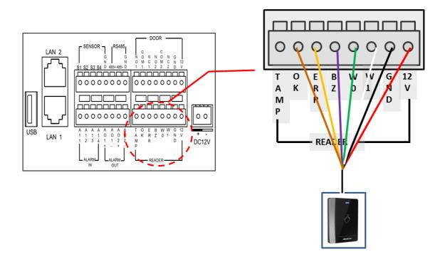
**Step 2:**Supply power to door station and issue card on door station or iVMS-4200 client, and test whether card reader works or not;
